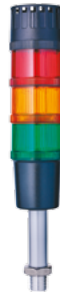
Order number: C70-Q641 Colours: red/orange/green Function: LED steady beacon, buzzer steady or pulsing tone Nominal voltage: 24 V AC/DC Type of mounting: horizontal Length: 100 mm
